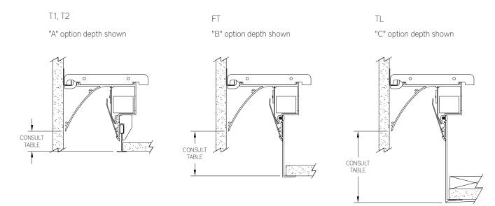
Three standard mounting depths above the ceiling plane are available. The measurement shown is the distance from the ceiling plane to the wall edge of the luminaire aperture.
