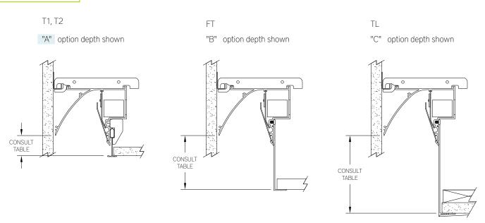
Three standard mounting depths above the ceiling plane are available. The measurement shown is the distance from the ceiling plane to the wall edge of the luminaire aperture.
