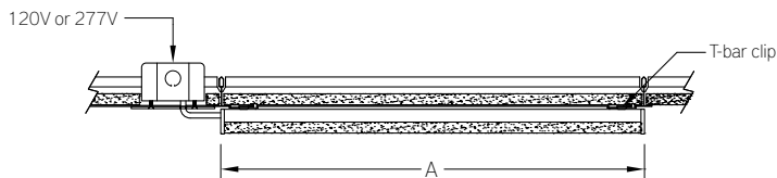
Side View - T-Bar Grid Ceiling Single Fixture
