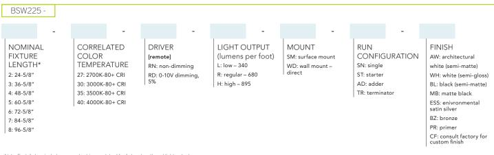
Note: Each fixture includes a remote driver matched for fixture length and light output. \* Actual dimension dependent on run configuration
