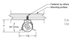
Each fixture is provided with one pair of screw mount spring clips. Use appropriate fastener through 5/32" hole.
