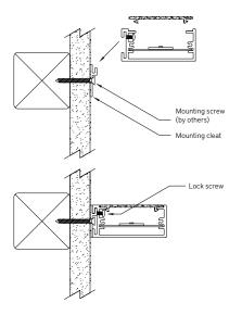
Use appropriate fastener through provided holes in the mounting cleat
