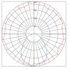
Maximun Candela = 255.9 Located at horizontal angle = 270 Vertical angle = 5 #1 - Vertical plane through horizontal angles (270 - 90) (through max. cd.) #2 - Horizontal cone through vertical angle (5) (through max. cd.)
