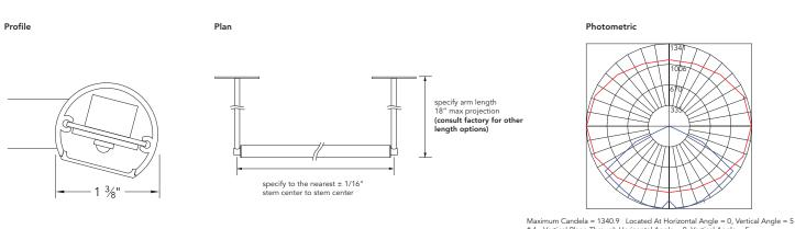
Maximum Candela = 1340.9 Located At Horizontal Angle = 0, Vertical Angle = # 1 - Vertical Plane Through Horizontal Angle = 0, Vertical Angle = 5 # 2 - Horizontal Cone Through Vertical Angle (5) (Through Max. Cd.)
